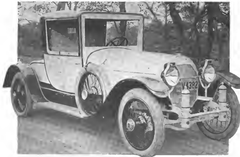
A typical custom-built body. This is a convertible roadster-coupe mounted on a Locomobile chassis
